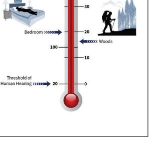
Noise Dose is the measured Sound Exposure Level normalized to an 8-hour work day. Exposure to sound pressure is regulated.
