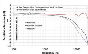
Free-field Response is the response of a microphone with respect to a single source normal to the microphone diaphragm in a free (nonreflecting) sound field.
