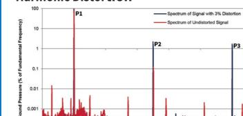
Total Harmonic Distortion (THD) of a system is the ratio of the root-mean-square sum of all of the powers of all of the harmonic frequencies to the power of the fundamental frequency.
